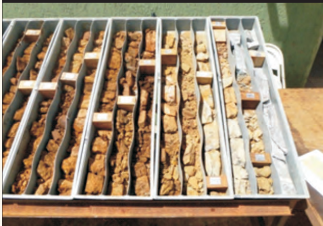
CORE LOGGING - SAPROLITE TO FRESH ROCK BOUNDARY
